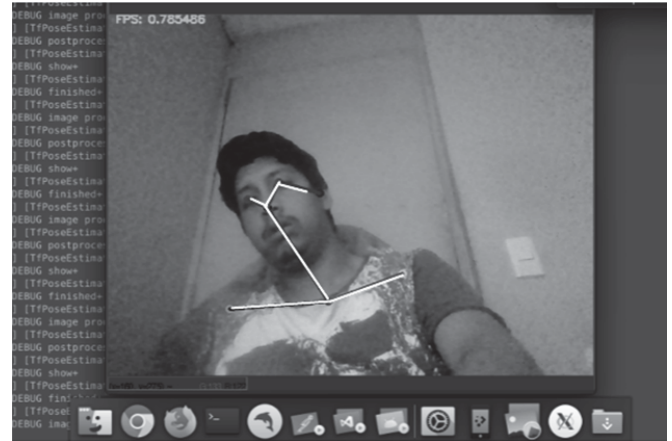
Fig. 7. Shoulder position estimation by OpenPose from a detected person
