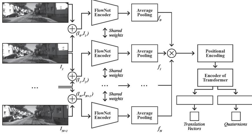
Fig. 1. The architecture of the proposed method for visual odometry. The dimensions of the tensors depend on input image size. Camera image credit: KITTI dataset [15].  $\oplus$  means concatenation over the channel,  $\otimes$  — stack of tensors.
