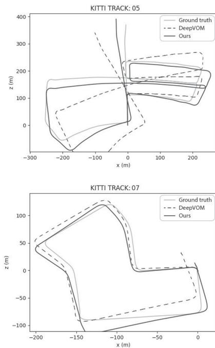
Fig. 2. Reconstructed trajectories of sequences 05 and 07 from the odometry benchmark of the KITTI dataset. [15]
