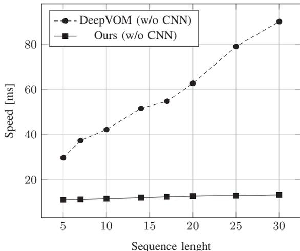
Fig. 3. Comparison of the speed of models at different sequence lengths running on the GPU of NVIDIA Jetson Nano.
