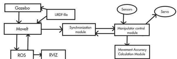
Fig. 2. Diagram of interconnections of software elements
