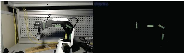
Fig. 4. Angles recognition on the manipulator with green labels
