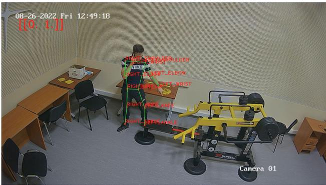
Fig. 4. Running the algorithm for recognizing human posture
