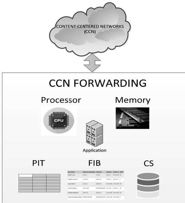
Fig. 1. Architecture of the components of a content-centric network
