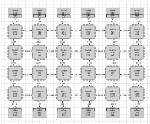
Fig. 5. The third diagram of a data transmission network with a 4x6-grid topology in SANDS
