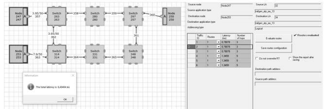
Fig. 8. The result of the modified method on the first network diagram with the "ring" topology
