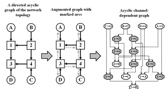
Fig. 1. The process of deadlock-free routes obtaining
