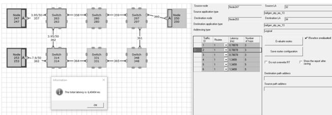
Fig. 6. The result of the basic method on the first scheme with the topology of the "ring" type network
