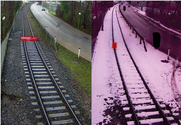
Fig. 4. Example images of obstacles that were detected highlighted by a red bounding box
