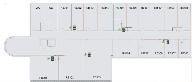
Fig. 1. Plan of KIS FRI UNIZA with the original location of AP We
