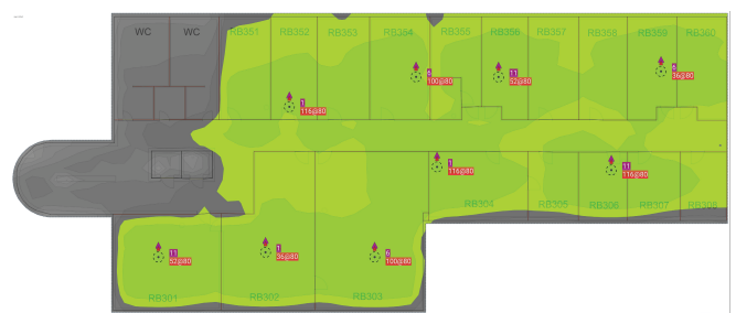
Fig. 10. Design of the AP position with an increased number of APs
