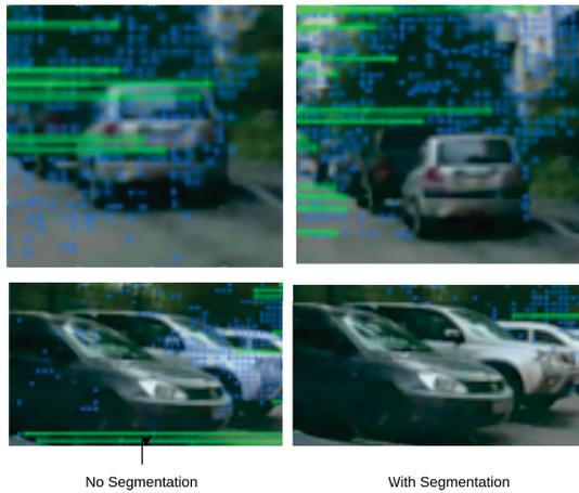
Fig. 7. Filtering the undesirable matching using segmentation on specific regions
