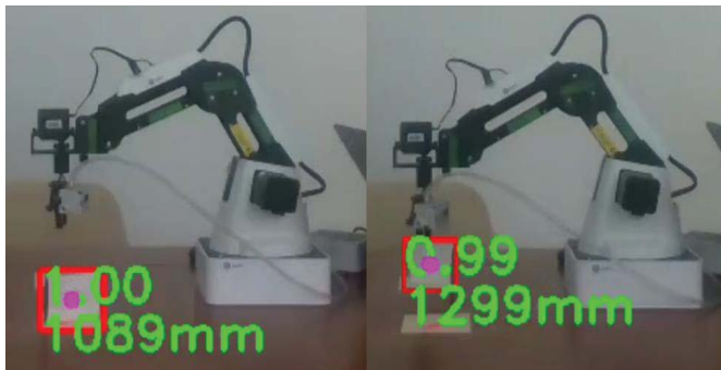
Fig. 1. Experiments with estimating the distance to the object being moved by the robotic arm: in the first position the distance is 1.089 m, in the second position 1.299 m
