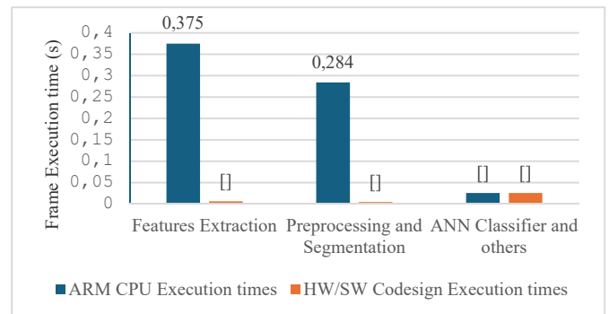
Fig. 9. Comparison of Execution Times Between HW/SW Co-Design and ARM CPU for Each Module
