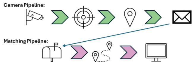
Fig. 4. This info graphic displays processes and connection between the two implemented pipelines. Every individual camera houses the camera pipeline, consisting in capturing, labeling, locating and transmitting data. A global matching pipeline is receiving such camera data, builds the trajectories by matching data and provides visualisation tools.
