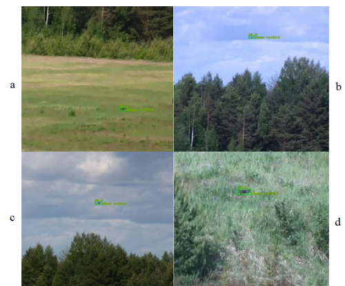
Fig. 7. Examples of frames from test videos where: a – object on a complex background (field), b, c – object on a simple background (sky), there is a brief flight of the object over the horizon line to a complex background, d – object on a complex background (field), there are moments when the object merges with the background
