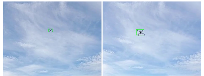
Fig. 8. Example of significant increase of object size. The object is on a simple background (sky) and has increased in size from 15*15 pixels to 40*30 pixels in 63 frames
