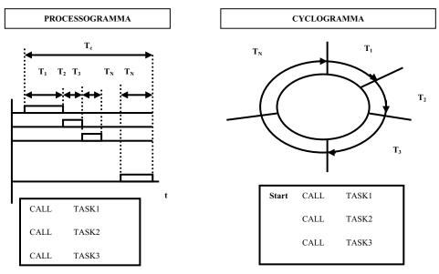
Figure 2.1. "Processogramma" and "Cyclogramma" illustration
