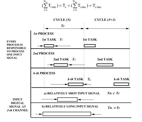
Figure 4.1 FIFO dispatcher processogramma
