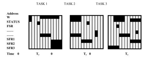
Figure 2.2 Examples of AT-maps W, STATUS, FSR, SFRx registers has unique numbers.
