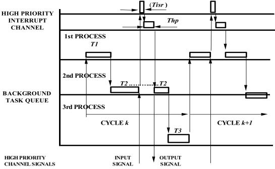
Figure 4.3 Processogramma for interrupt-based system
