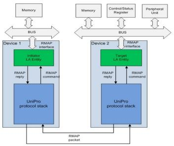
Figure 4. Initiator and Target LA Entity function
