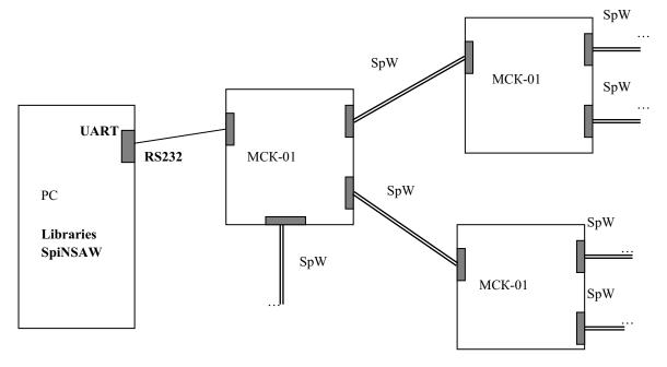
Figure 5. Example of SpaceWire network
