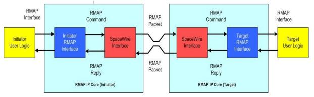
Figure 1. RMAP IP Core Data Flow
