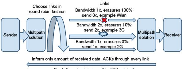
Fig. 1. General architecture of the FEC-multipath
