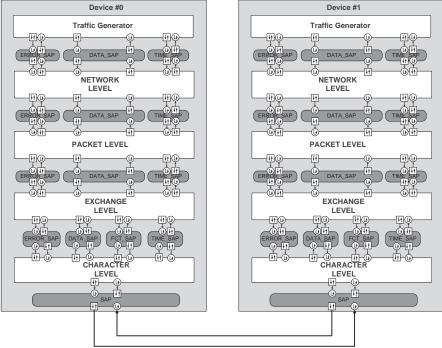
Fig. 5. An example of SpaceWire point-to point modelling case
