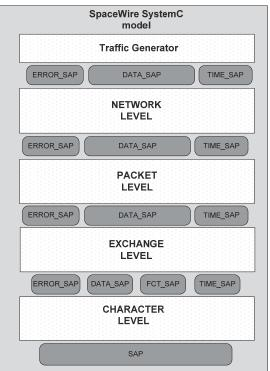
Fig. 3. SpaceWire SystemC model architectural diagram
