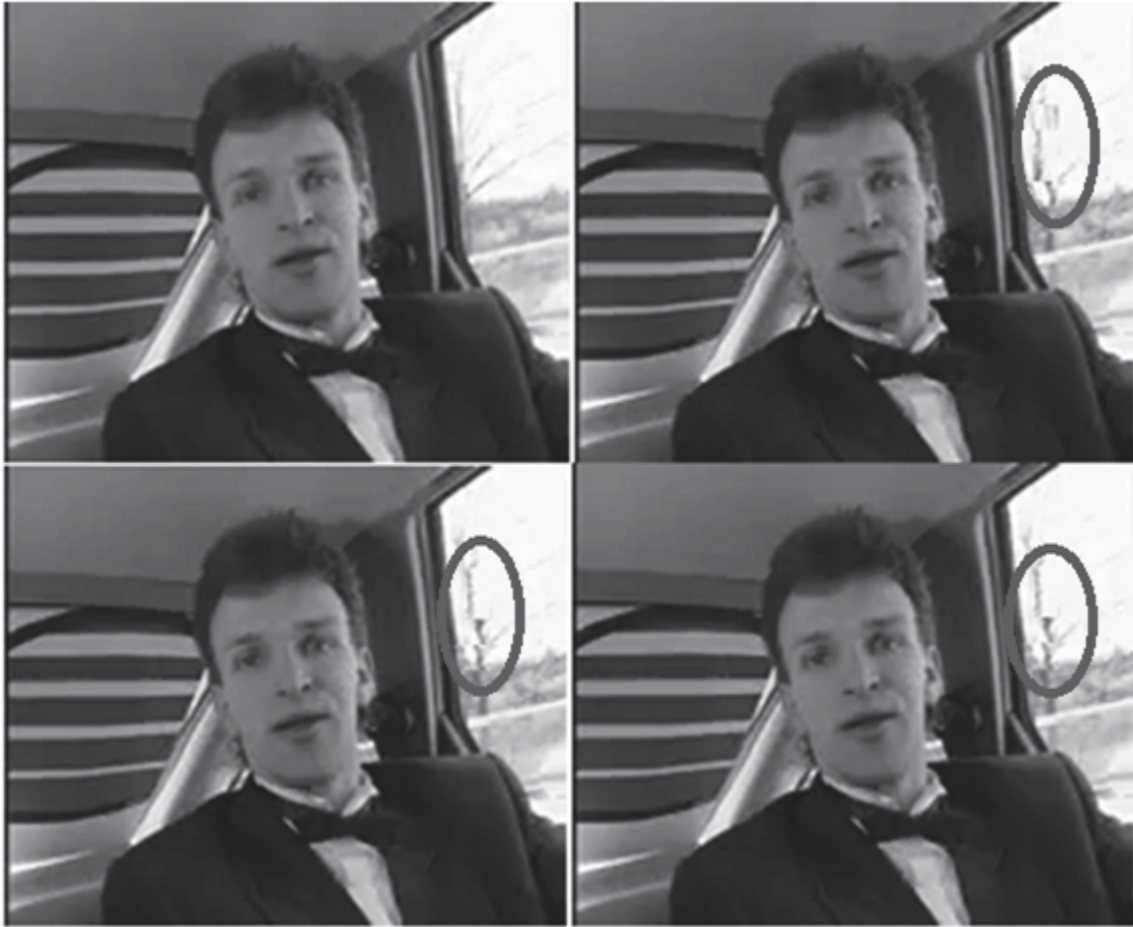
Fig.4. Restored Frames by FFT-based method with different levels L. Top-left – initial frame; Top-right – L1; Bottom-left – L4; Bottom-right – L10.
